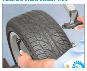
Inner and outer Dataset® Arms speed entry of wheel data and placement of clip-on or adhesive weights while increasing accuracy and allowing single-spin balances.
