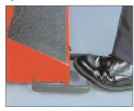
Tapping the foot brake activates entry and storage of wheel data. Foot pedal also locks spindle for easier tightening and loosening of wing nut.
