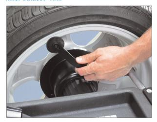
Inner Dataset® Arm determines exact placement for weights. Automatically measures wheels up to a 28" diameter.
