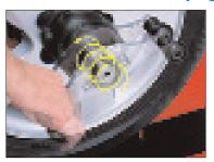
With a double tap of the foot pedal, the ServoDrive™ system feature automatically takes up unused spindle threads, eliminating hand cranking of the wing nut.
